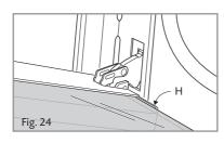
The top oven door has a sealed gasket in the top part.
